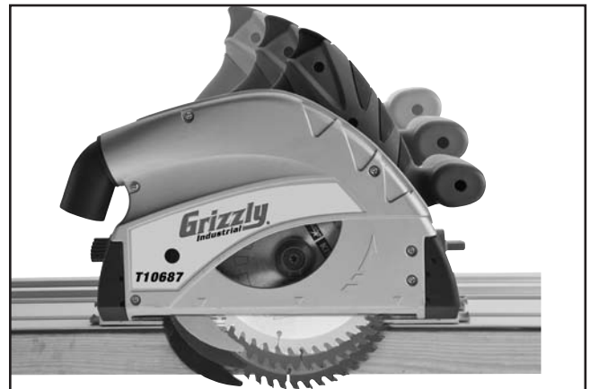
Figure 20. Plunge-action lowering for the cut.
